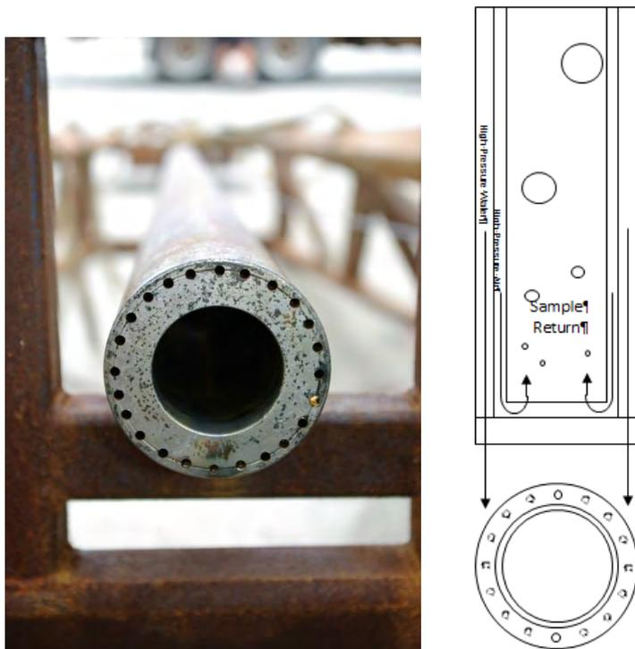
Figure 2 Cross sections of a reserve circulation drilling tube
