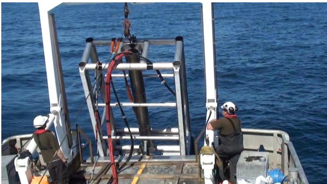
Figure 1 Launch of the drill rig from the vessel
